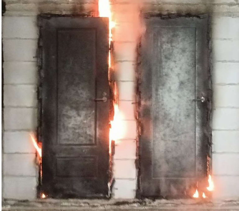
Fig. 5 Exposed Side after 20 Minutes
