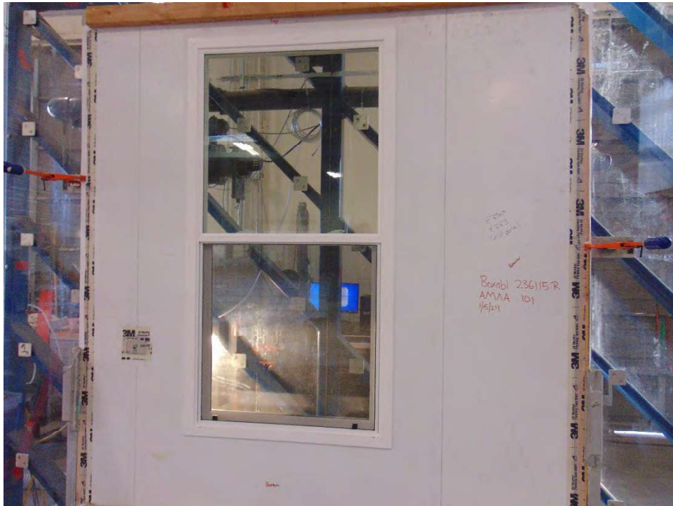
Photo 2: ASTM E283 Total Leakage Measurement
