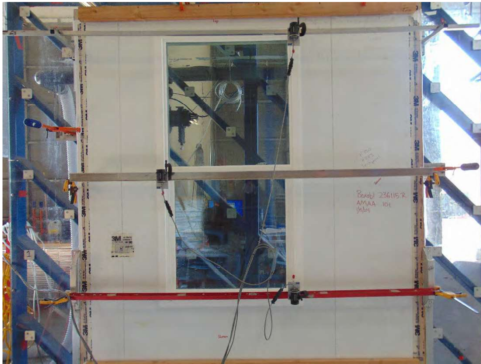
Photo 3: Uniform Load Deflection Measurement
