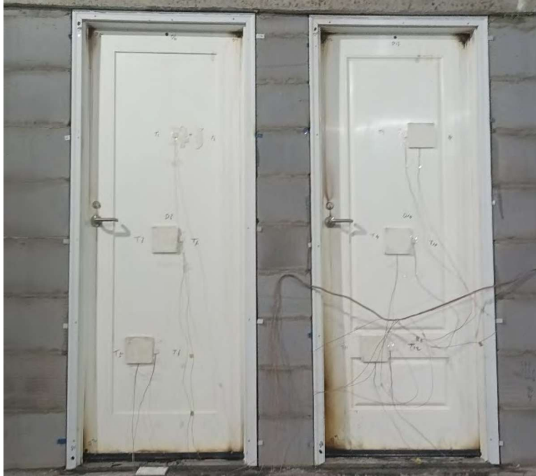
Fig. 7 Unexposed Side after Hose Stream Test
