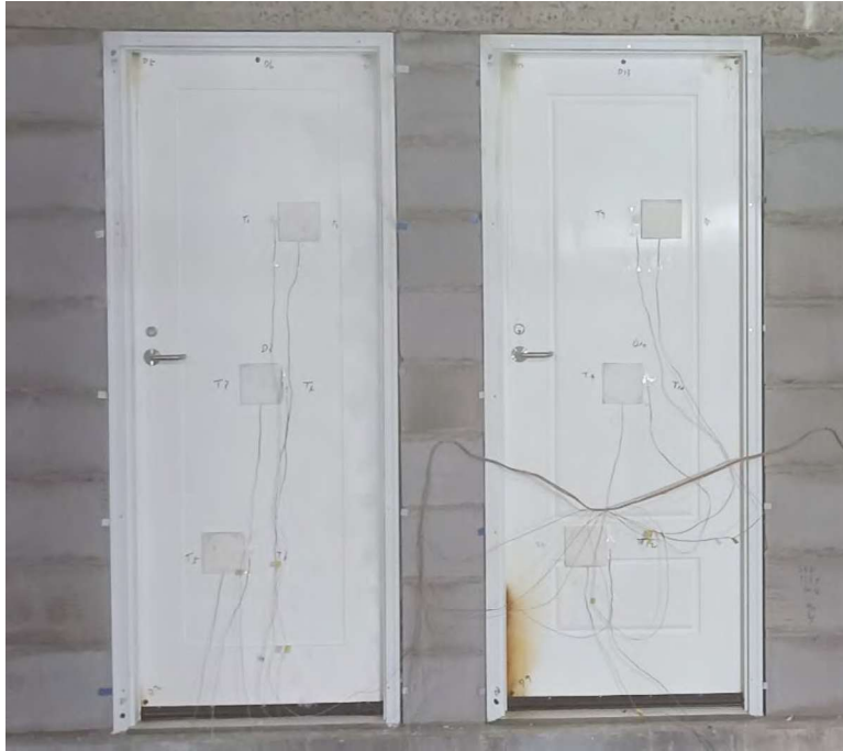
Fig. 3 Unexposed Side after 10 Minutes
