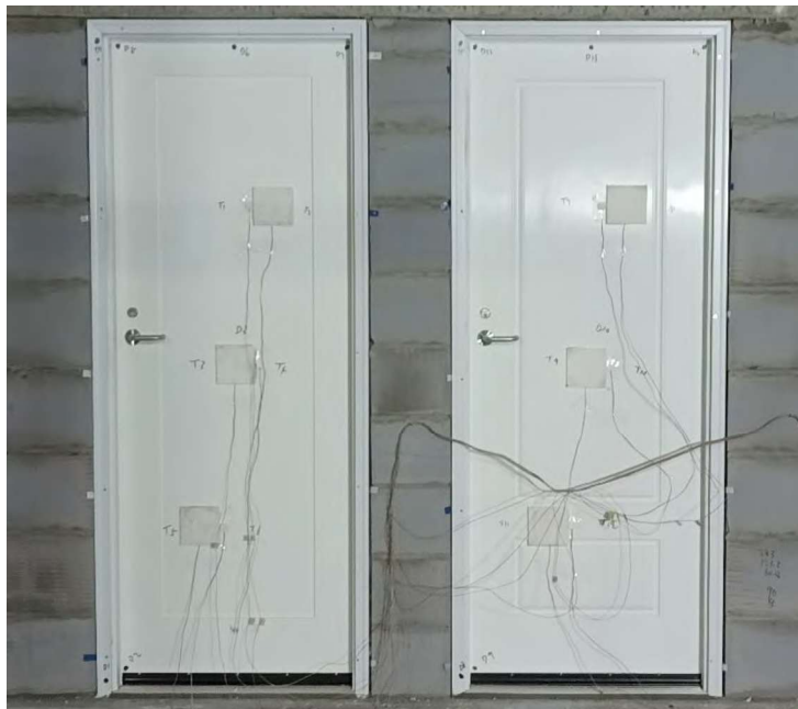
Fig. 2 Unexposed Side Prior to the Fire Test
