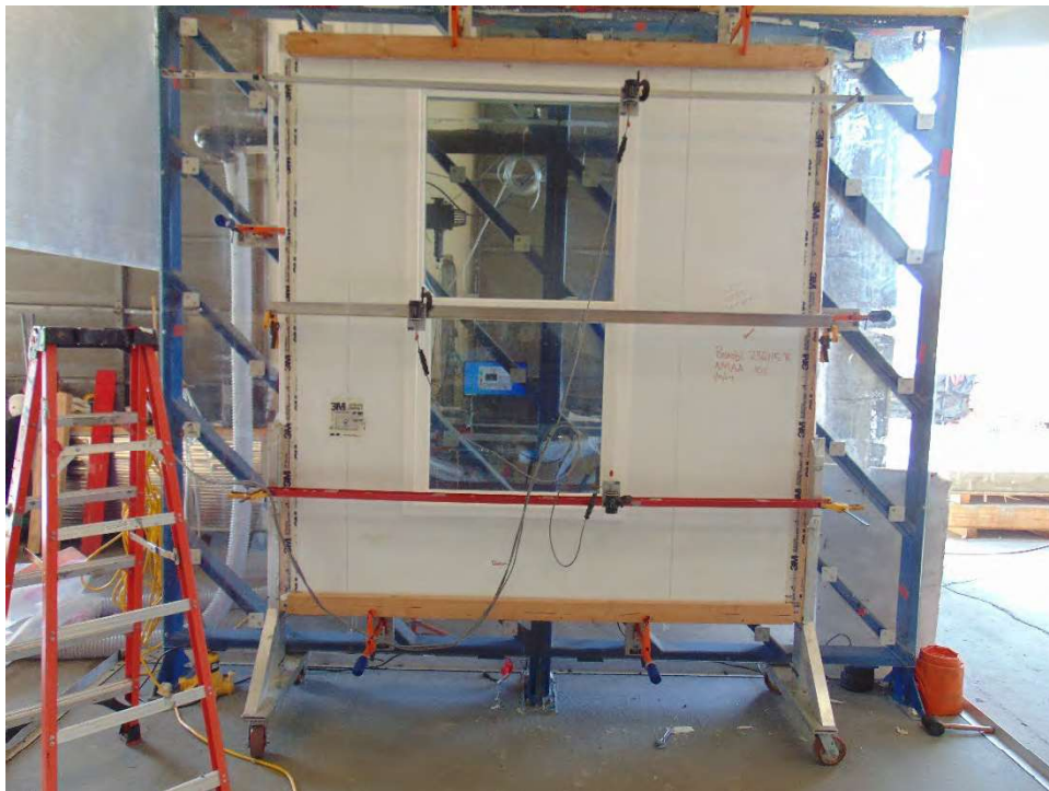
Photo 4: Structural Loading, per ASTM E330
