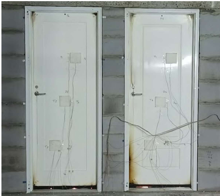
Fig. 4 Unexposed Side after 20 Minutes
