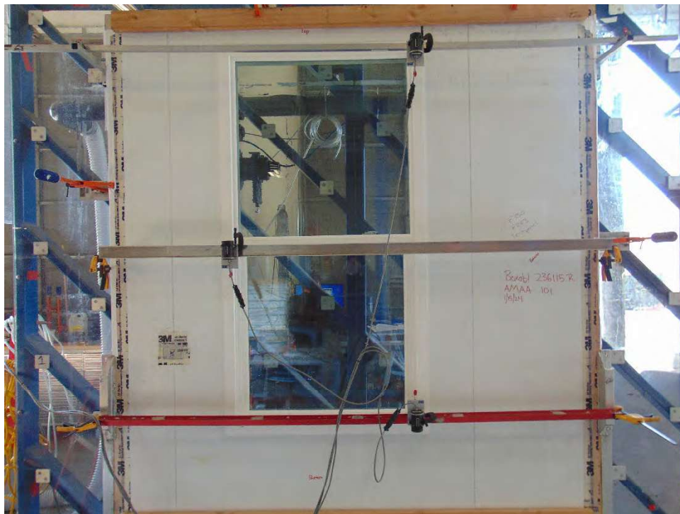
Photo 3: Uniform Load Deflection Measurement
