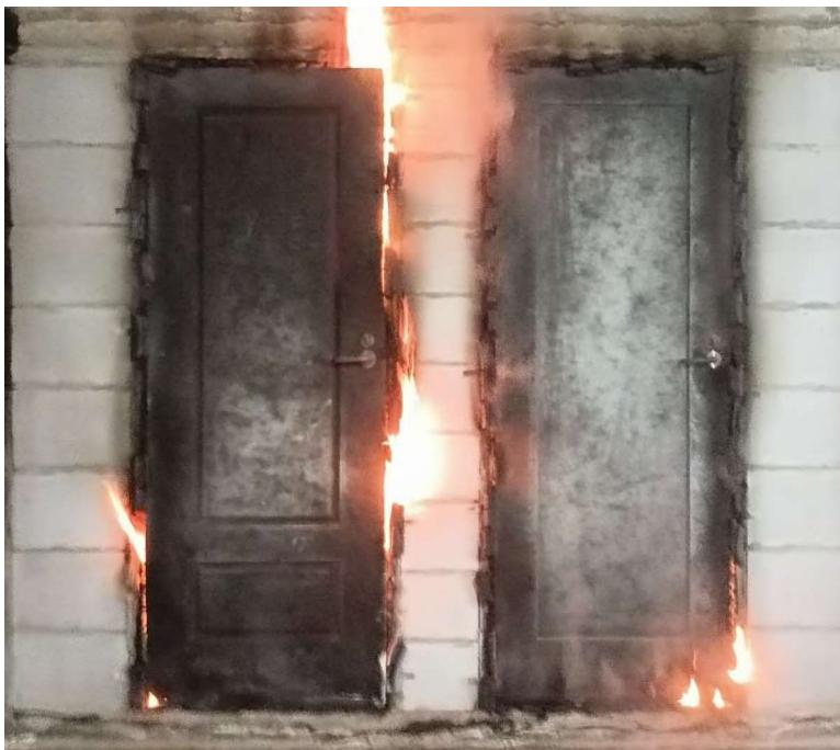
Fig. 5 Exposed Side after 20 Minutes
