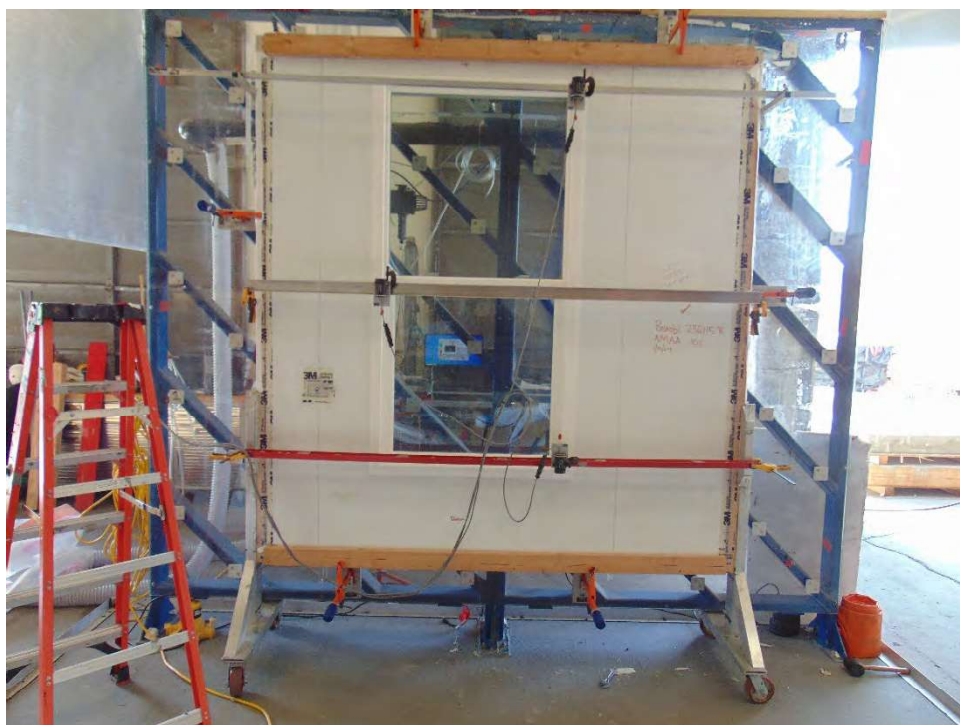
Photo 4: Structural Loading, per ASTM E330
