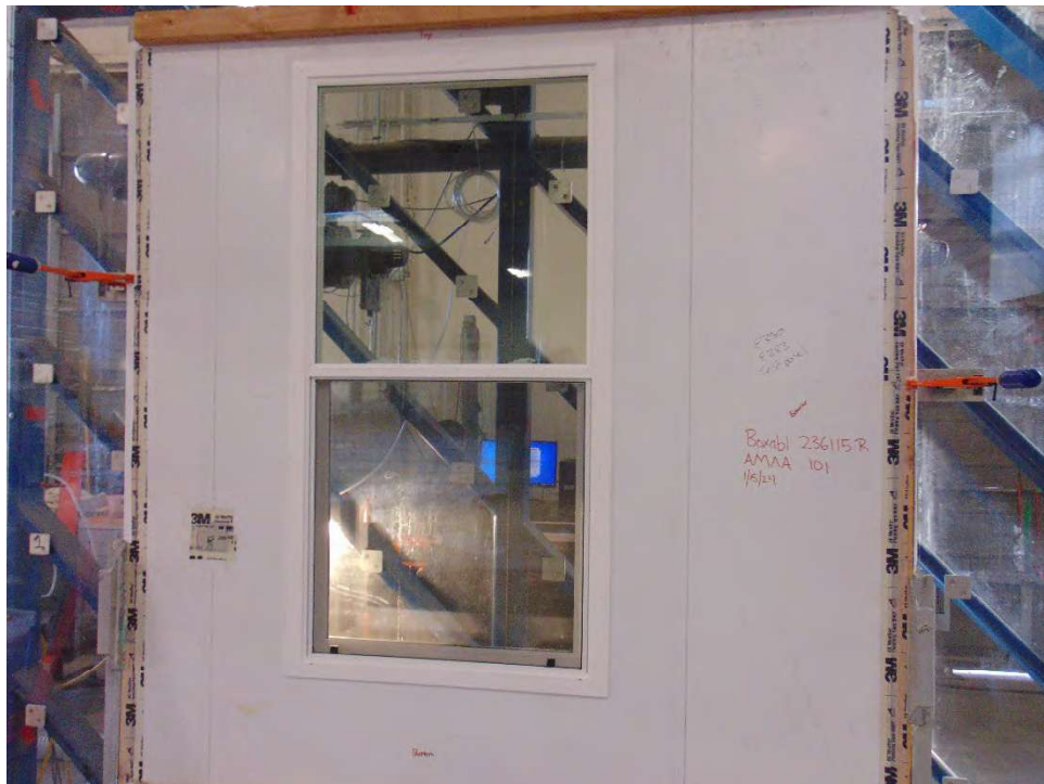
Photo 2: ASTM E283 Total Leakage Measurement
