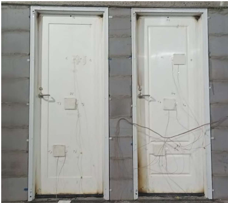
Fig. 7 Unexposed Side after Hose Stream Test
