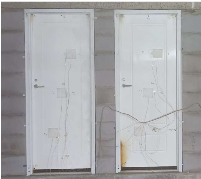
Fig. 3 Unexposed Side after 10 Minutes
